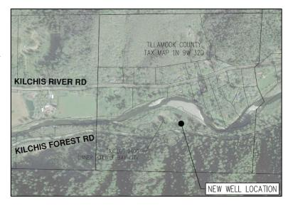
The project seeks approval to develop a 3<sup>rd</sup> well on Tax Lot 2400 owned by Bay City. The well is to be added as SRC-AC under their existing entry point (EP-A), receiving the same treatment as wells #1 (SRC-AA) and #2 (SRC-AB) provided at their existing treatment plant (WTP-A). See page 7 of this letter for more details.
