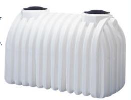
All Norwesco cistern tanks are manufactured by means of the rotational molding process, which produces a one-piece, seamless, watertight tank. Polyethylene is unaffected by soil chemicals so Norwesco the tanks will not rust or corrode and require no additional coatings as other tanks do. Norwesco's strict quality guidelines ensure an environmentally safe cistern tank.
