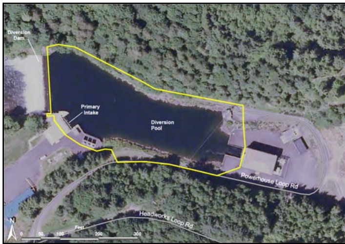
Figure 3. Inspection Area for the Diversion Pool Perimeter and Drainage Systems
